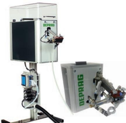
Sword feeders or segment feeders are used when the requirement calls for gentle, almost noiseless feeding of sensitive fasteners. Our sword feeder systems can process screw sizes from M2 to M6. They are ideal for screws up to 25 mm in length. Sword (segment) feeders are also well-suited for the processing of balls and pins.
