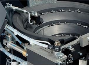
DEPRAG feeders with a vibratory drive are particularly suitable for screws from < M1 to M8. Shaft lengths of 5 mm to 50 mm can be processed. For counter-sunk head screws especially, vibratory bowl feeders are a functional solution. The high output of DEPRAG vibratory bowl feeders distinguishes them from other feeding systems.
