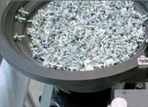
If feeding via a hose system is not possible e.g. if the screw has a non favourable ratio in relation to the head diameter vs overall length, then we offer special solutions such as a pick-and-place procedure with vacuum pick or gripper pick devices.
